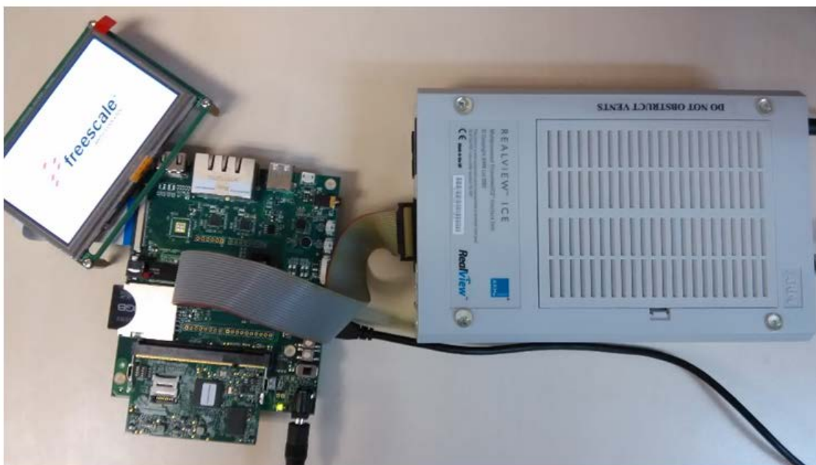
Figure 4. i.MX 6UL-EVK connection with RealView-ICE Debugger
